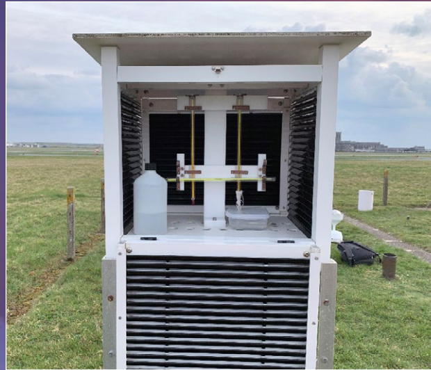
Interior of Stevenson screen showing thermometers
